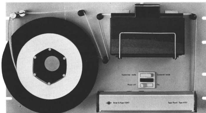
Fig.3.2. Correct Threading of Paper Tape through Tape Handler
